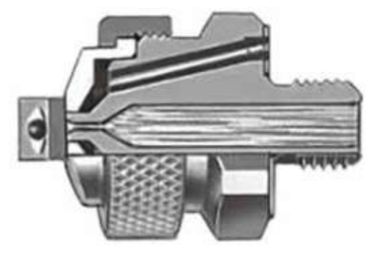
External mix with pressure set-ups: flat spray patterns
